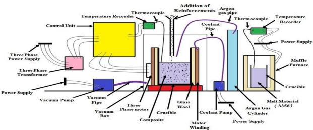
Fig: 1. Schematic View of Electromagnetic Stir Casting Set-Up
