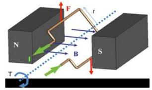
Fig: 1. Schematic Diagram of a Coil of Wire Conduction Current in a Magnetic Field
